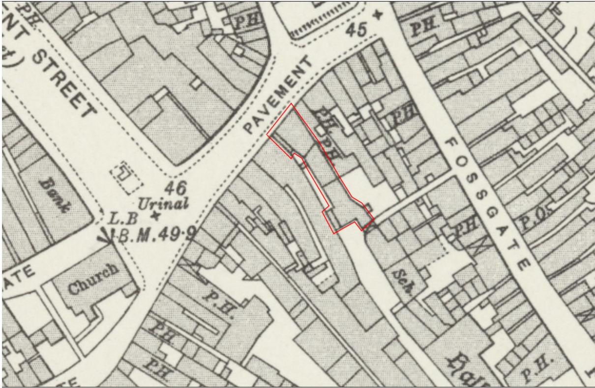
Plate 9 Detail of 1909 OS 1:1250 map, site in red. Note the loss of the external stair and complete infilling of the courtyard between Buildings A&B (© Crown Copyright).
