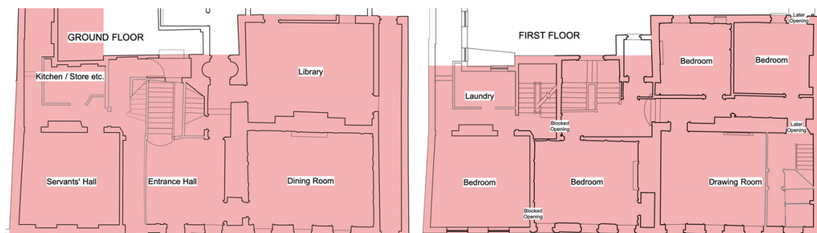
Fig. 4.7 Current ground & first floor plans of nos. 29-31 with 1835 footprint (red), and original room labels added based on dimensions. Later walls within the 1835 plan are shown as grey dotted lines.
