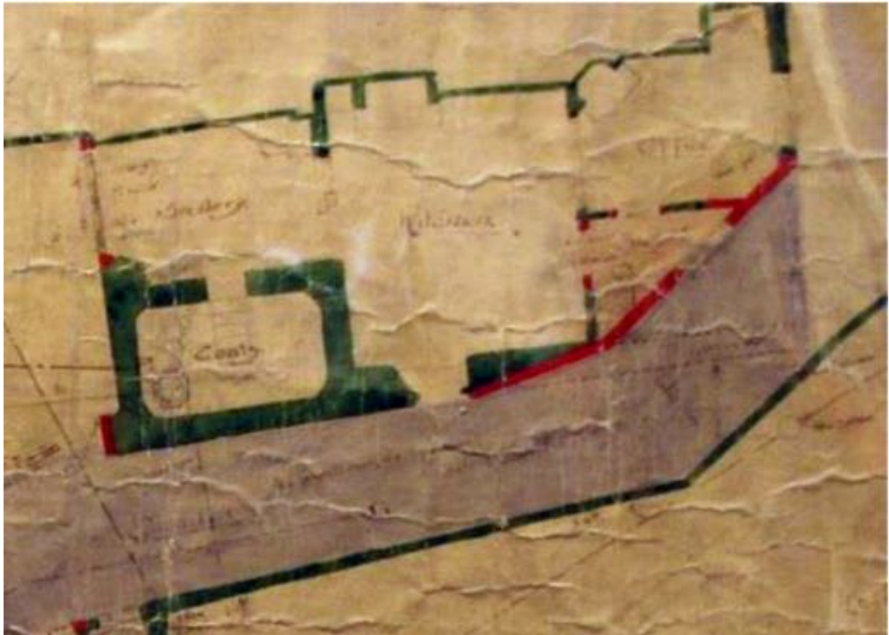
Fig. 2.10 1901 Ground Floor Plan by Frank A Tugwell, ARIBA, showing the changes to the angled ground floor recess in TWH (new 1901 work shown in red) © YorkExplore Archives
