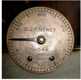
Above: The setting dial, an essential aid for adjusting the time on the external hands, is also a traditional place for the maker's name and year of manufacture.
