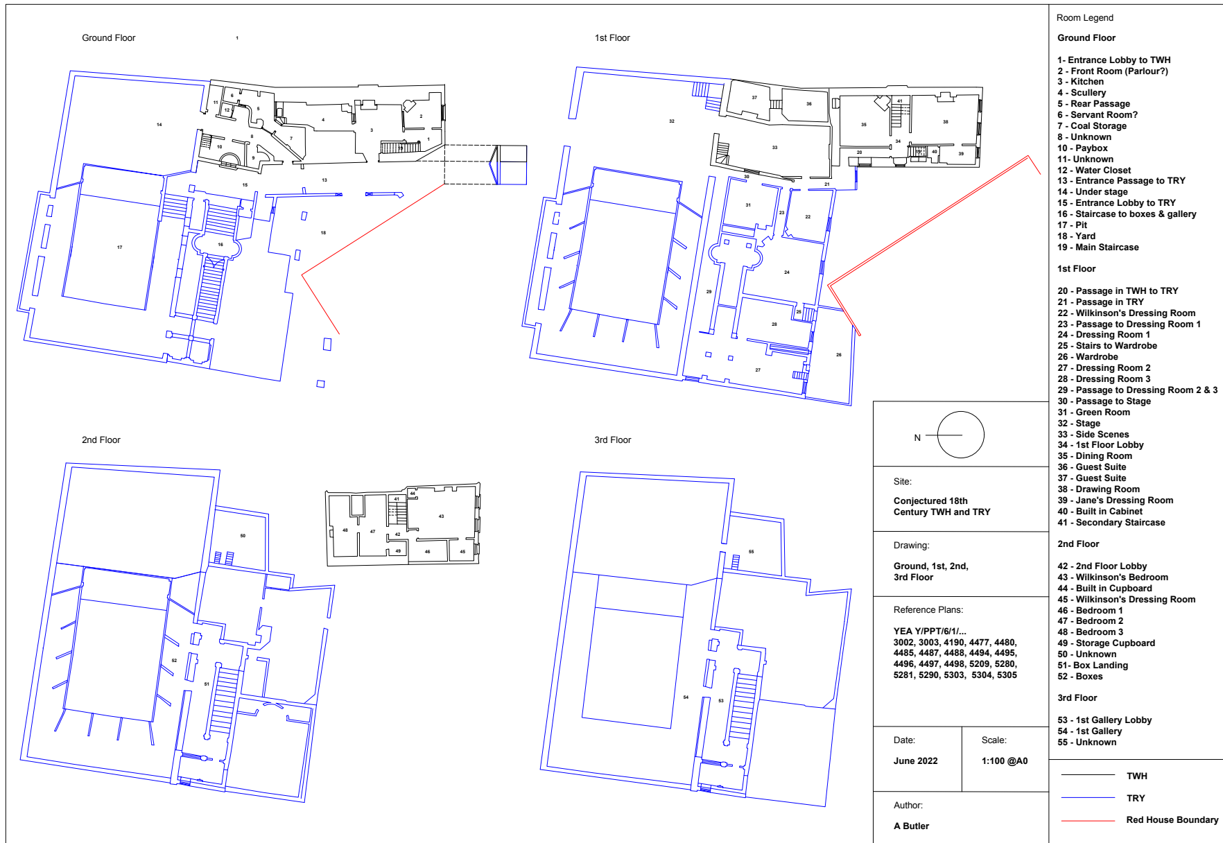
Figure 31: Access map of the TWH and TRY (top) based on 18 th century conjectured floor plans (bottom) (Author 2022).
